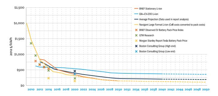
FIGURE 2 Lithium-Ion Battery Prices Have Declined Sharply and Are Expected to Continue Declining
